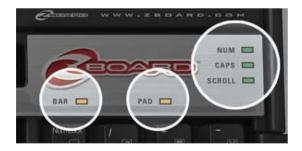
In addition to the LED indicators you would find on a traditional keyboard for Caps Lock, Scroll Lock and Num Lock, the Zboard<sup>TM</sup> has three LEDs to support some of its unique functions, including an Enabled LED (which indicates the Zboard<sup>TM</sup> Keyset is working properly when the application is active – see "Enabled LED"), and Pad and Bar LEDs to indicate when the functions in those areas are active.
