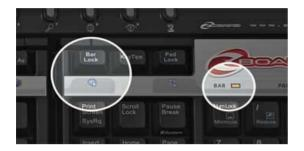
NOTE 1: When the Bar LED is illuminated, indicating that the Bar Area is active, standard function key (F1 - F12) operations are not available. To enable the standard function key features, press the Bar Lock key to disable the "Internet Bar" Area.
