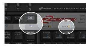
NOTE: When the Pad LED is illuminated, indicating that the Pad Area is active, the standard number and navigation key functions are not available. To enable the traditional numerical keypad features, press the Pad Lock key to disable the Pad Area. Pad Lock over-rides Num Lock.
