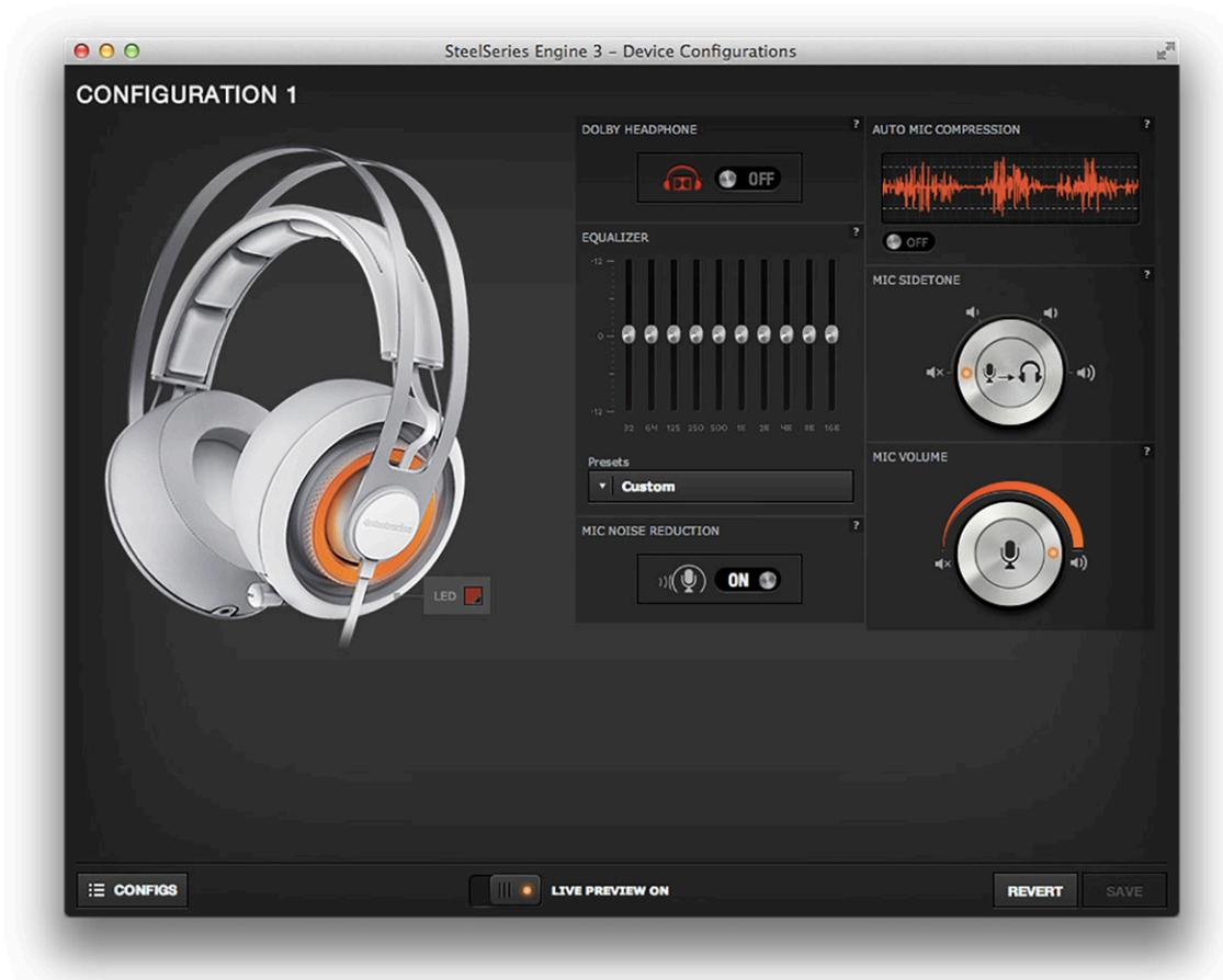
*Siberia Elite's* configuration window includes unique widgets for customizing LED lighting, sound quality, and microphone settings.
