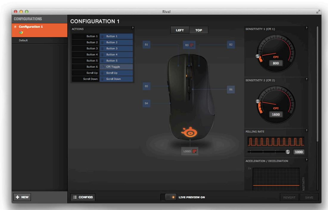
*Rival's* configuration window includes widgets for customizing mouse sensitivity, mouse/computer communication, and auto-correction for horizontal and vertical paths.
